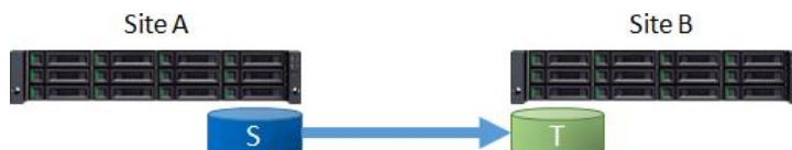
Figure 12-22 One-Directional Remote Replication
