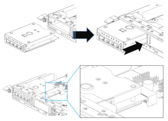
Figure 3-13 Procedures of Installing the Host Card
