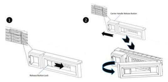
Figure 3-2 Unlock and Open the Carrier Handle of a Disk Drive Tray (LFF)
