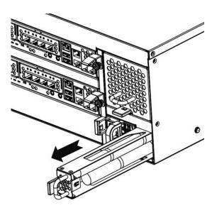
Figure 6-25 The Procedure of Removing the Power Module from the System Chassis
