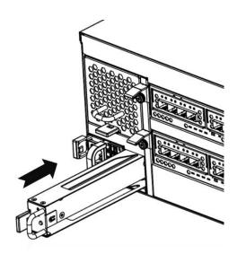
Figure 3-20 Installing the Flash Module
