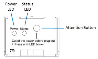
Figure 6-23 Pressing Attention Button of the Flash Module
