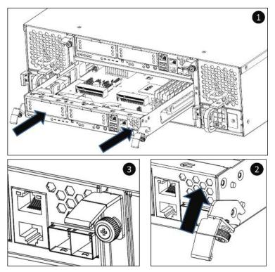
Figure 6-5 Detailed Procedures of the Controller Module installation
