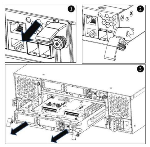
Figure 3-11 Steps of Removing the Controller Module
