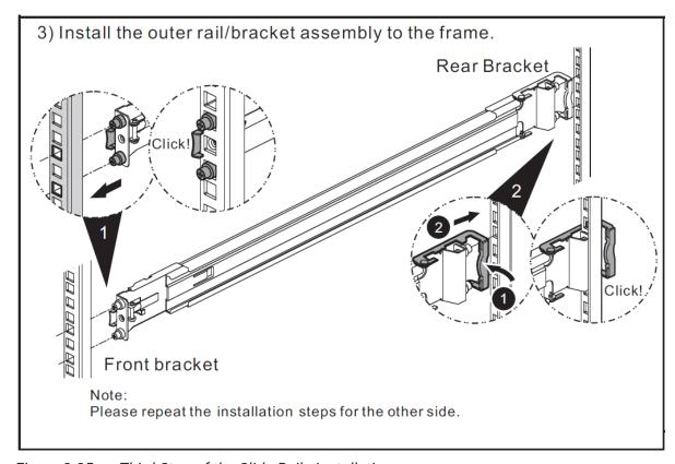
Figure 3-25 Third Step of the Slide Rails Installation
