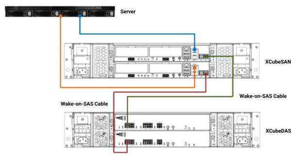
Figure 3-31 One Server / One HBA / One XCubeSAN / One XCubeDAS / Dual Path
