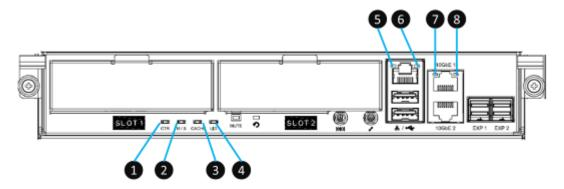
Figure 5-3 The Controller LEDs
