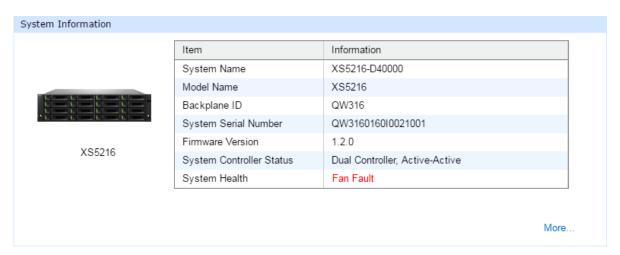
Figure 6-12 Warning Message of Failed Fan Module in the SANOS UI
