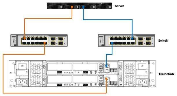
Figure 4-3 One Server / One HBA / Two Switches / One XCubeSAN / Dual Path
