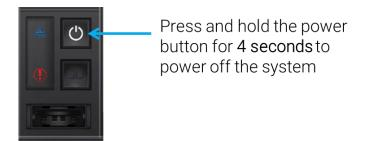
Figure 3-34 Power off the System by Power Button
