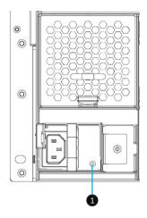
Figure 5-4 The Power Supply Unit LED
