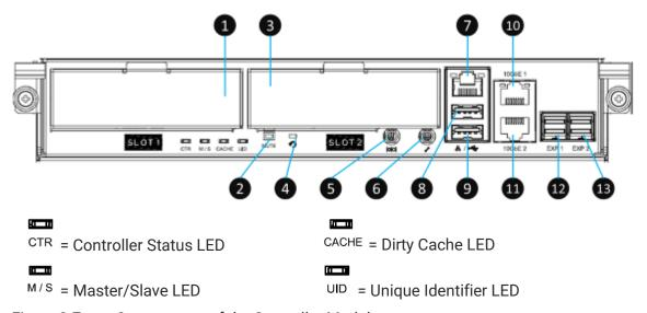
Figure 2-7 Components of the Controller Module
