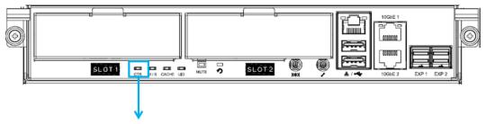
If controller status LED shows solid red, it means the controller module encounters some sort of issues or hardware configuration mismatch.
