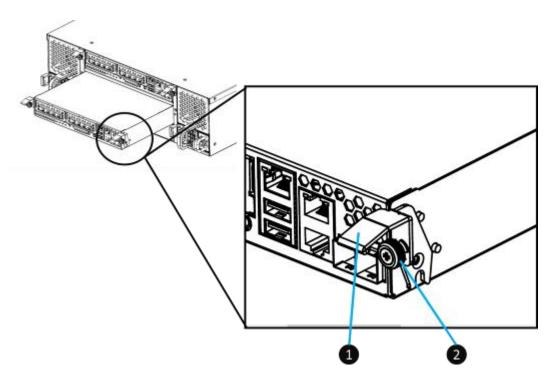
Figure 3-10 Mechanical Components of the Controller Module
