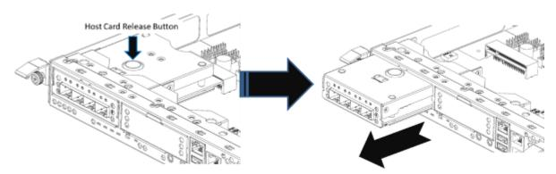
Figure 6-18 Procedures of Removing the Host Card from the Controller Cage
