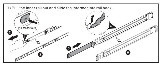
Figure 3-23 First Step of the Slide Rails Installation
