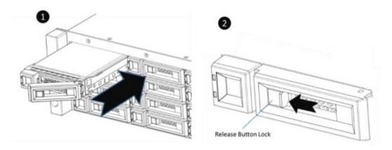
Figure 3-27 Install a Tray into the System and Lock the Release Button Lock (LFF)
