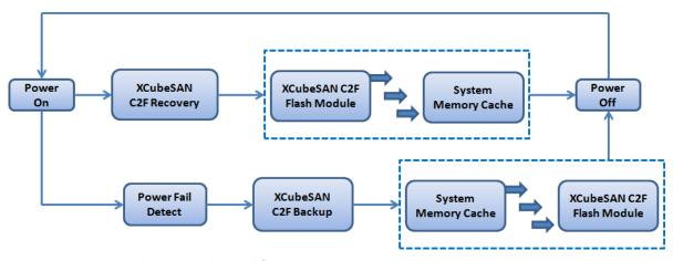
Figure 2-15 Cache-to-Flash Workflow
