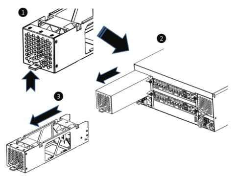
Figure 6-14 Procedures of Removing the Fan Module
