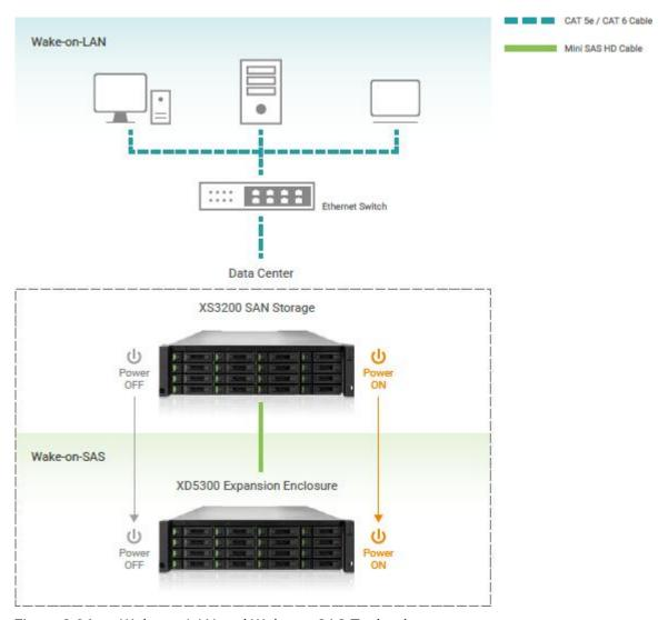
Figure 3-36 Wake-on-LAN and Wake-on-SAS Technology
