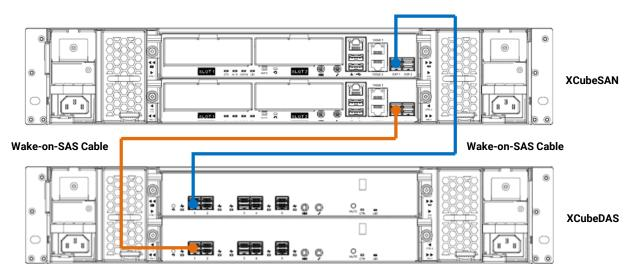
Figure 4-8 Cascade Topology: One XCubeSAN / One XCubeDAS / Dual Path
