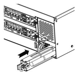
Figure 3-21 Installing the Power Module
