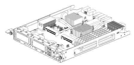
Figure 2-6 General View of the Controller Module
