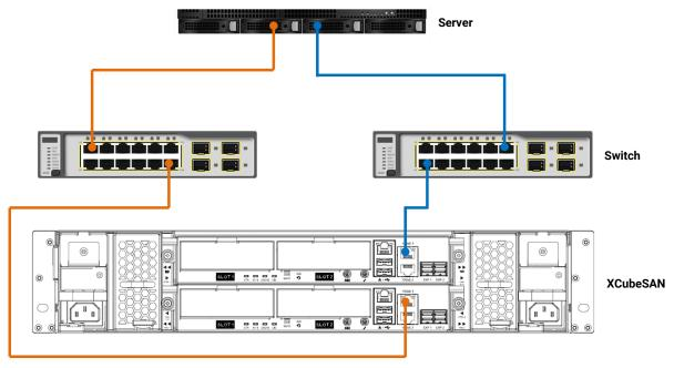
Figure 3-30 One Server / One HBA / Two Switches / One XCubeSAN / Dual Path
