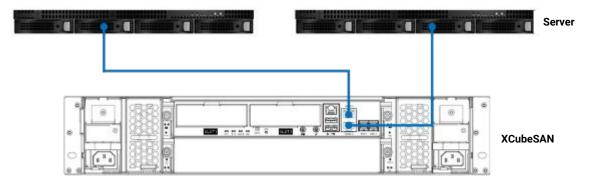
Figure 4-5 Two Servers / One HBA per Server / One XCubeSAN / Single Path
