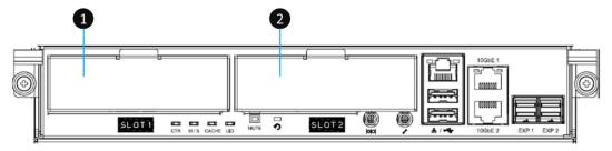
Figure 3-9 Host Card Installation Slots
