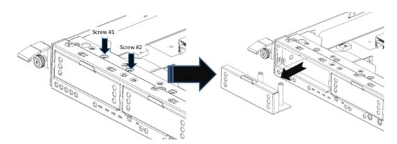
Figure 3-12 Procedures of Removing the Host Card Dummy Cage
