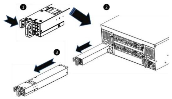
Figure 6-9 Procedures of Removing the Power Supply Unit
