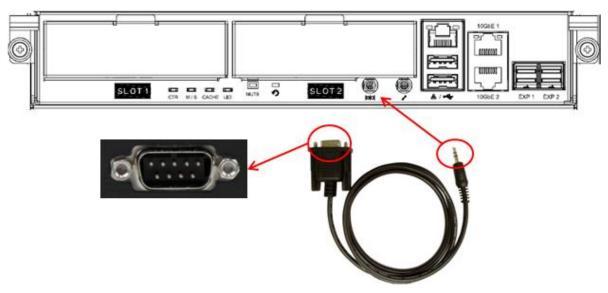
Figure 7-3 Connect the Console Cable
