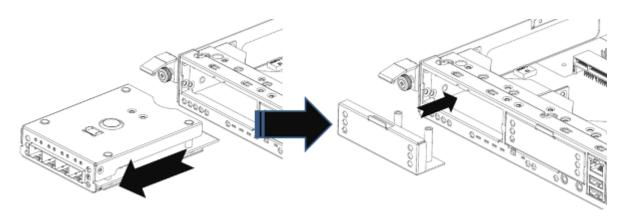
Figure 6-19 Procedures of Pull out the Host Card and Install Dummy Host Card Cage
