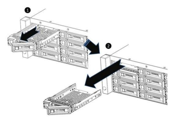
Figure 3-4 Hold the Carrier Handle and Pull out the Disk Drive Tray (LFF)
