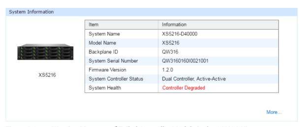
Figure 6-1 Warning Message of Failed Controller Module in the SANOS UI
