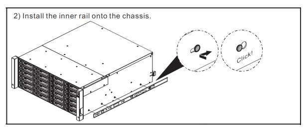
Figure 3-24 Second Step of the Slide Sails Installation
