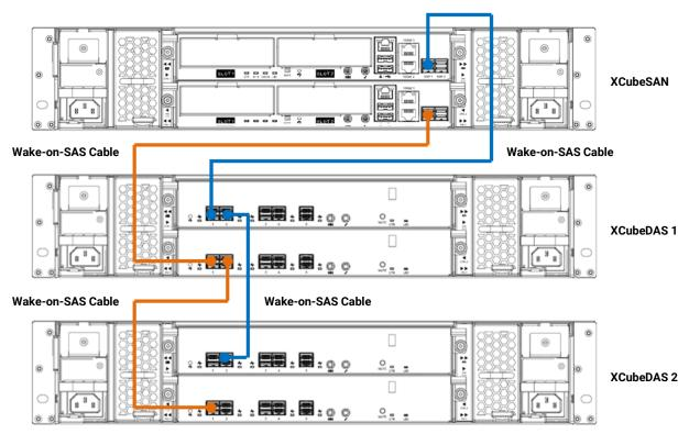
Figure 4-9 Cascade Topology: One XCubeSAN / Two XCubeDAS / Dual Path
