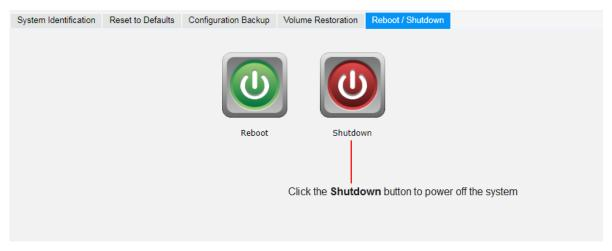
Figure 3-35 Power off the System via Web UI
