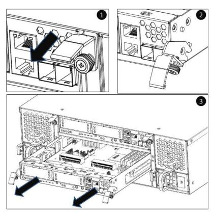
Figure 6-4 Procedures of Removing the Controller Module
