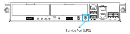
Figure 3-37 Location for the UPS System Connection
