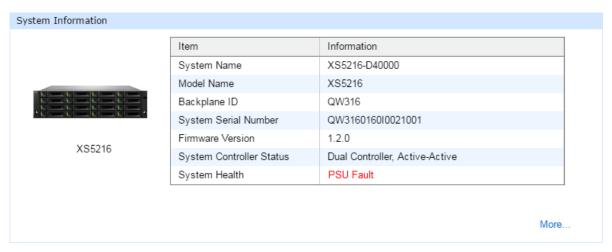
Figure 6-7 Warning Message of Failed PSU in SANOS UI
