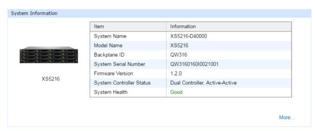
Figure 6-6 Screenshot of the Controller Module Successfully Installed in SANOS UI
