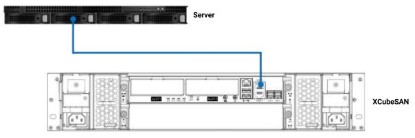
Figure 4-1 One Server / One XCubeSAN / Single Path
