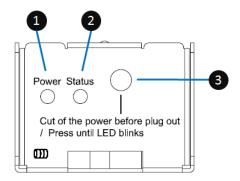
Figure 5-10 Flash Module LEDs and Button
