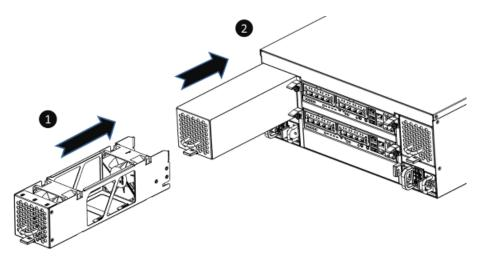
Figure 6-15 Procedures of Installing the Fan Module
