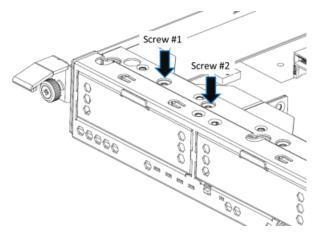
Figure 6-20 The Finished Installed Dummy Host Card Cage
