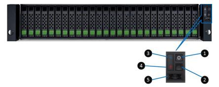
Figure 2-1 System Controls and Indicators
