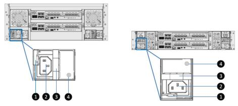
Figure 2-8 Power Supply Unit Components
