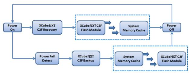
Figure 2-14 Cache-to-Flash Workflow
