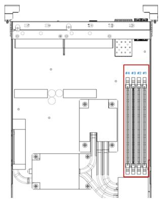
Figure 3-1 Memory Module Slot Number
